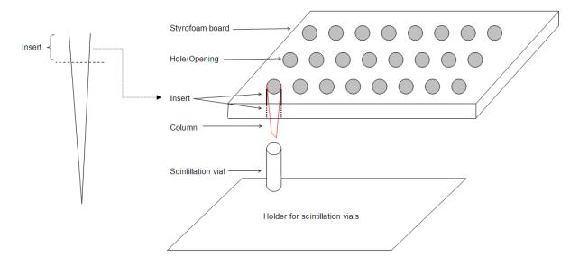
The Styrofoam containers for disposable cuvettes work nicely as scintillation vial holders. Keep in mind that most scintillation cocktails dissolve Styrofoam.
